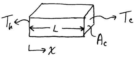
$$\dot{q} \propto \frac{\Delta T}{L} A_c \quad \Delta T = T_h - T_c$$
